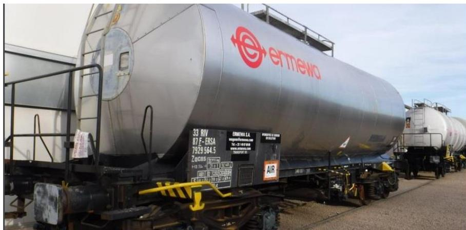
The 4-axle rail tank (Zacns) car with a capacity of 50 m<sup>3</sup> is designed for the transport of **Sodium Hydroxide**. The wagon complies with the latest European legislations in force.
